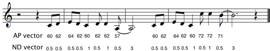
Fig. 2. An example of the representation of the melody of the song “ From me to you ” ( The Beatles ) using the AP (absolute pitch) and NV (note value) vectors.
