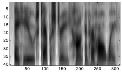
The original spectrogram is reproduced by resampling the result above. Note the fine lines indicating the pitch have been lost by the MFCC process. This is a useful feature for speech-recognition systems since they want a representation that is blind to pitch changes.
