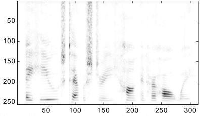
After combining several FFT channels into a single mel-scale channel, the result is the filter bank output. This is shown below (the fb output of the mfcc command includes the  $\log 10$  calculation.)
