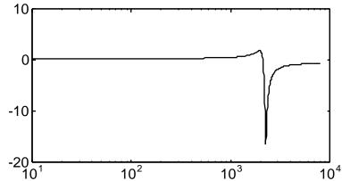
Then the gain of the filter section is set to 10 (20dB) near the filter's best frequency (1960 Hz). The new frequency response is plotted below.
