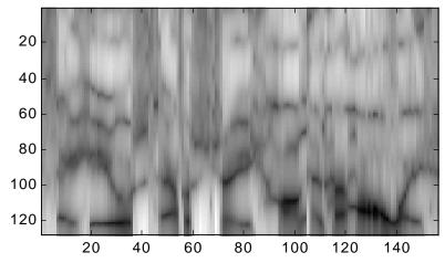
The spectrogram for LPC with a 26th order polynomial is shown below. Note how there is more detail in the spectrogram, because a 26th order polynomial can capture more details in the spectrum within each frame.
