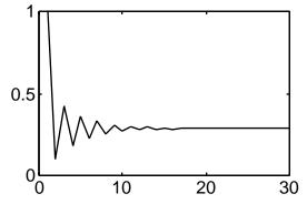
Finally, we switch to a much longer time constant (smaller value of epsilon.) This makes the response much less likely to oscillate, but now the AGC takes longer to cut the signal level to the target.
