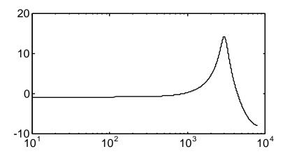
Likewise, a simple band-reject filter is formed by using a pair of zeros. The resulting filter looks like this.
