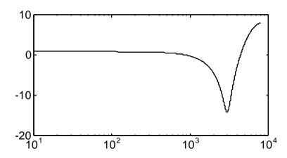
A broader filter is formed by using a lower q, in this case 2. \*sos=SecondOrderFilter(3000,2,16000)
