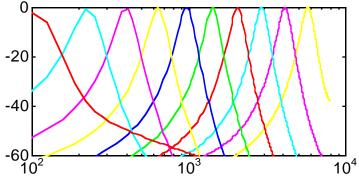
A simple cochlear model can be formed by filtering an utterance with these filters. To convert this data into an image we pass each row of the cochleagram through a half-wave-rectifier, a low-pass filter, and then decimate by a factor of 100. A cochleagram of the 'A huge tapestry hung in her hallway' utterance from the TIMIT database
