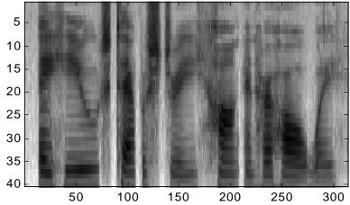
Finally, the conversion into the cepstral domain uses the discrete cosine transform to reduce the dimensionality of the output. We can invert the cosine transform to get back into the filter bank domain and see how much information we have lost. The *recon* output is shown below (flipped again so that the high frequency channel is at the top). Note the result is much smoother then the original filter bank output.
