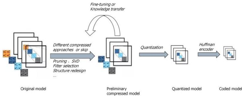
**Figure 7 - Framework for neural network compression.**
