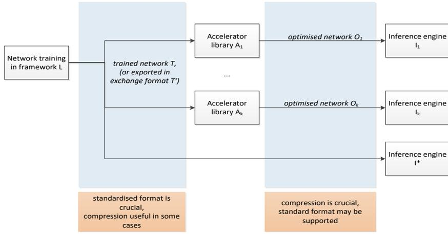
**Figure 6 - Deployment/inference process.**
