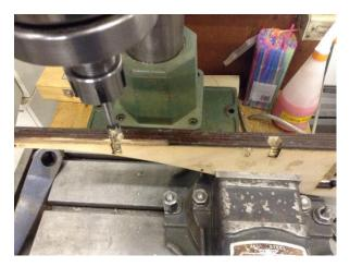
Now the wood has to be sanded and polished (if required) for a smooth finish. The lower wooden frame (PT-2-1) can be screwed to the Aluminium frame. All the 2.5mm holes must be tapped to M3 threads for the Perspex to be mounted. The Ply-wood is now screwed into the lower wooden frame.
