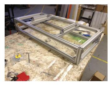
Once the main frame has been constructed the work can start on the long linear rails. The mountings and housings for the 8mm chromed slider rods and the housing for the Potentiometer and bearings are all 3D printed for ease of manufacturing but could feasibly be cast or milled in Aluminium. These are mounted to the hollow Aluminium square section with M6 steel bolts and to the frame
