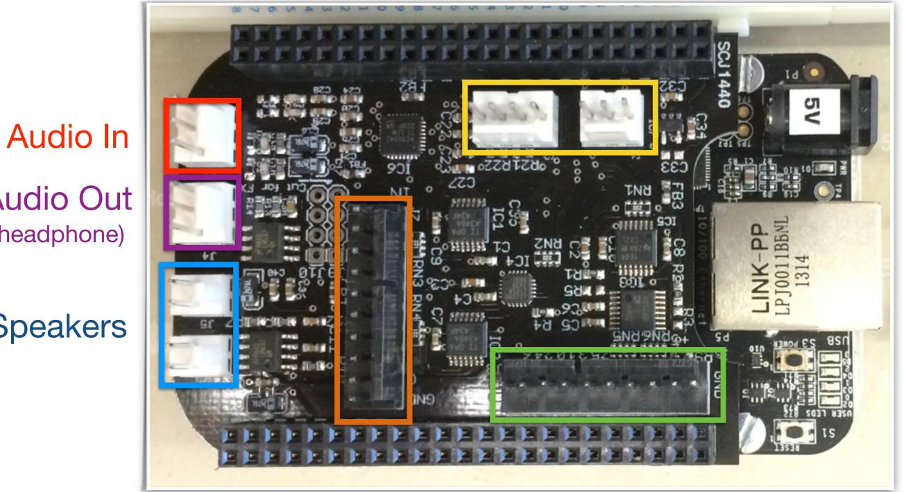
8-ch. 16-bit ADC 8-ch. 16-bit DAC
